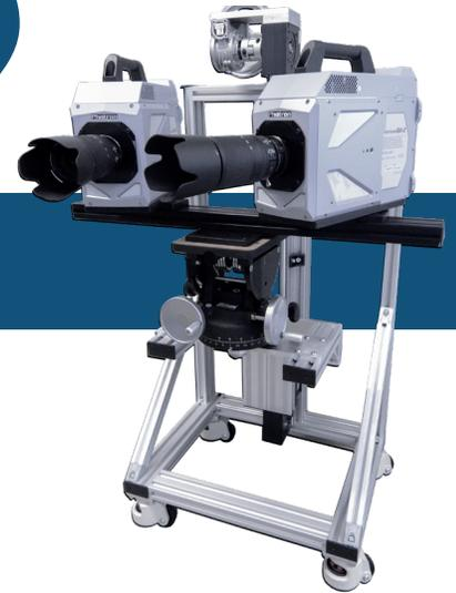
The VIC-3D system from Correlated Solutions is the most powerful turn-key system for non-contact measurement of full-field surface shape, deformation, strain, vibration, and much more. With a range of new features including direct data comparison of FE mesh data and a new graphics engine called *iris*, which can produce extremely high-resolution still and moving images, the VIC-3D system is poised to change the way engineers around the world validate models and share their results.
